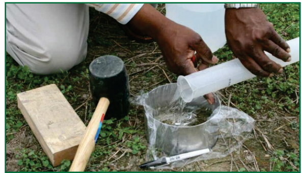
Figure 2.—Water is poured into plastic-lined ring.
